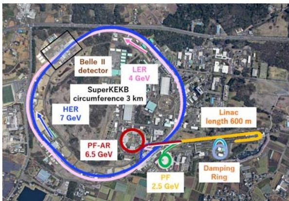
Figure 1: Schematic layout of KEK e<sup>+</sup>/e<sup>-</sup> Linac and related accelerators.
