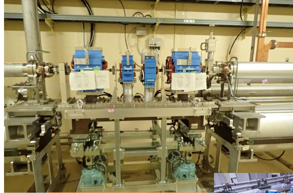
New pulsed magnets QF Horizontal steering Vertical steering QD
