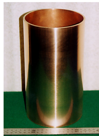
Figure 2: Cu/Nb/Cu clad seamless pipe made by cladding, hot&cold rolling, deep-drawing and spinning.
