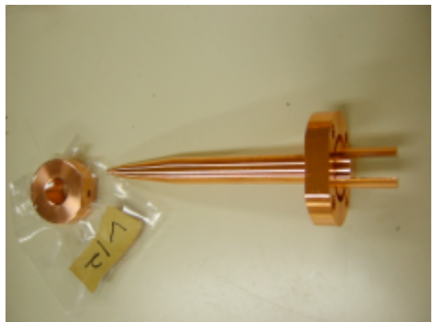
Fig7. Photograph of the manufacturing cavity Fig8. Photograph of Drift tube and stem
