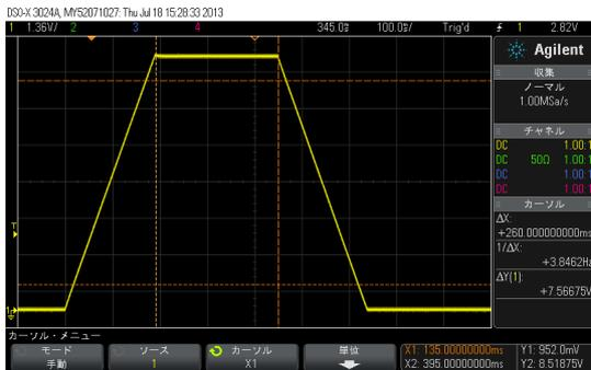
Figure 2: The pulse current of BM-LS (in pattern-mode). The rise time and fall time are 190 ms, and the pulse width on the top is 260 ms.
