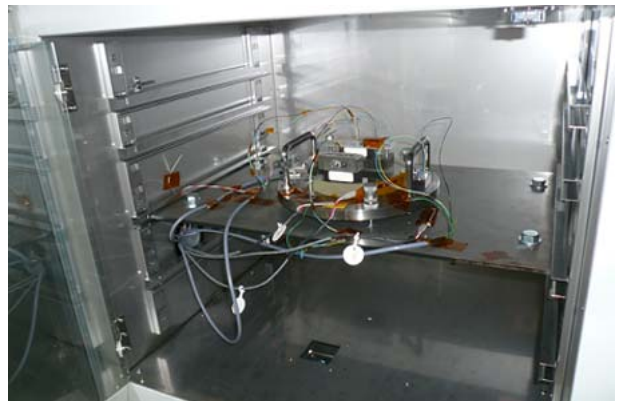
Figure 1: Tilt sensors in the regulated temperature box.
