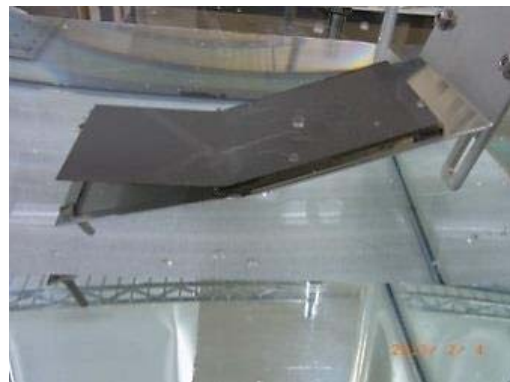
Figure 3: A photo of a support jig for a foil separation from glass substrates.
