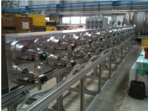
Figure 4: Photograph of real size aluminum RFQ module; the axial length of 9.78m-long.
