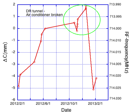
Figure 5: Change of the circumference during 2012~2013, which is estimated from the change of the DR acceleration frequency
