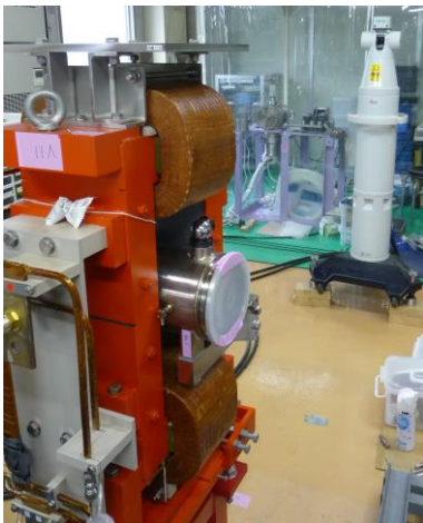
Figure 6: BPM Alignment at test bench.
