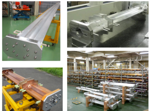
Figure 4: Antechamber-type beam pipes.
