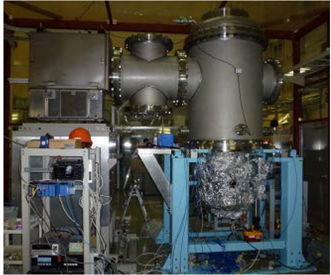
Figure 1: Cross section view of the 2nd 500 kV photocathode DC-gun (left) and a photograph of this system (right).
