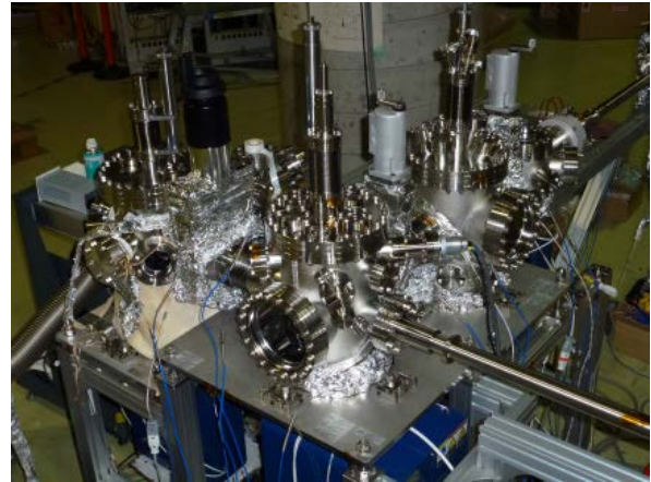
Figure 8: Schematic view of the cathode preparation system with functions of simultaneous plural cathodes cleaning, activating and storage (left), and a photograph of this system without a vacuum suitcase (right).
