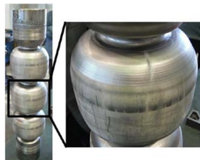
Figure 6: Ruptured pipe after hydroforming process
