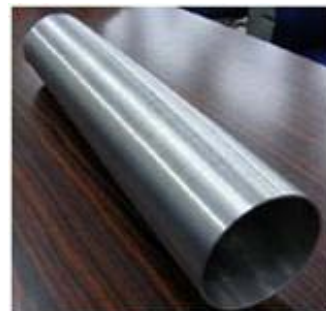
Figure 1: Seamless Nb pipe for 3-cells cavity
