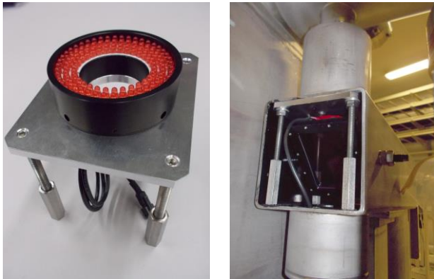
a) The ring-type LED light with a bracket b) LED light in the blind duct
