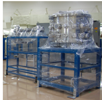
Figure 14: Photograph of the irradiation test equipment for space-use devices (S4 line).
