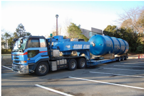
Figure 2: Transportation of the accelerator tank by a heavy equipment trailer truck.
