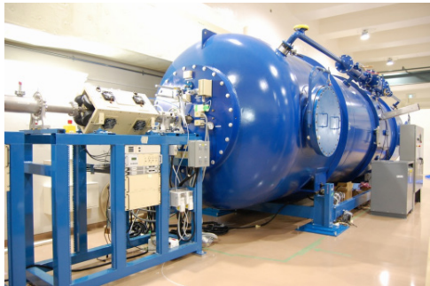
Figure 6: Photograph of the 6 MV tandem accelerator tank at the accelerator room (August, 2014).
