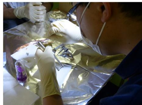
Figure 5: Replacing a cathode of injector linac.
