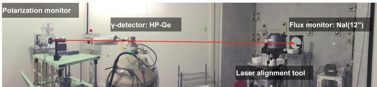
Figure 2: Experimental setup of LCS gamma-ray spectra measurements at GACKO, gamma-ray irradiation hutch 2 at NewSUBARU.
