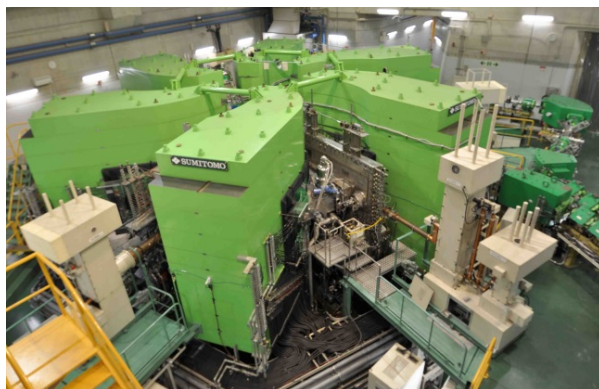
Figure 1: A whole view of the ring cyclotron at RCNP. FT cavity, its power feeder, and the amplifier cabinets are seen from the center to the lower right in the picture.
