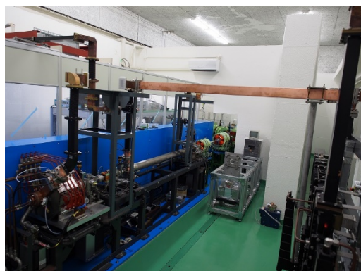
Figure 1: Layout and photo of S-band RF gun based accelerator facilities at ISIR, Osaka University.
