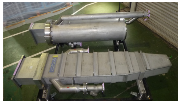
Figure 1: High-power water-loads (upper: cylindrical-type, under: rectangular-type).
