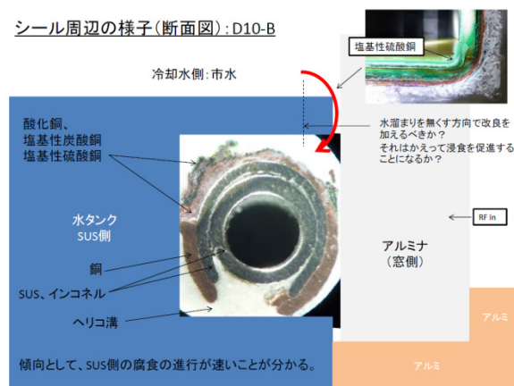
Figure 6: Example of a cross section of the metal seal and the structure around metal seal.
