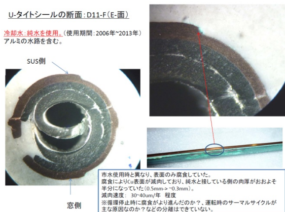
Figure 7c: Cross section of a corroded metal seal (D11-E, pure water, E-plane).
