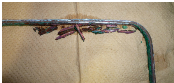
Figure 3b: Corrode of metal seal (D10-B, tap water).
