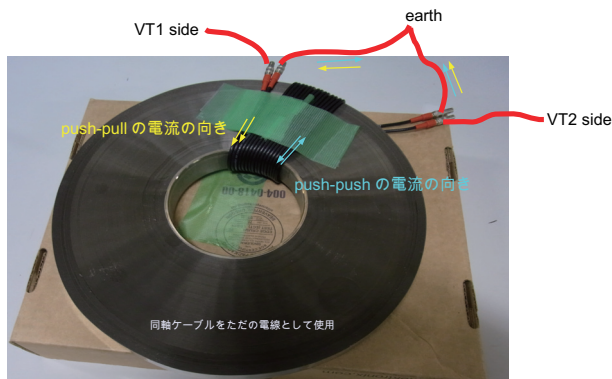
Figure 1: The operating principle of the MA balun. This is a low power balun using coaxial cables as normal cables.
