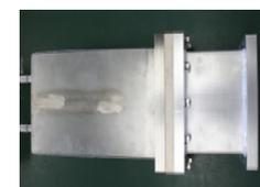
Figure 12: Circulator, water load.
