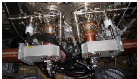
Figure 11: Coupler of Main Linac.
