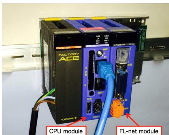
Figure 1: PLC data acquisition system via FL-net.
