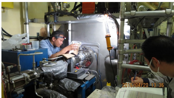
Figure 3: Photograph of the work for a leakage of insulation vacuum chamber in superconducting vertical wiggler.
