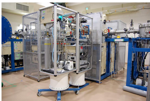
Figure 5: Photograph of the CO 2 Gas Type MC-SNICS and the Injection System.
