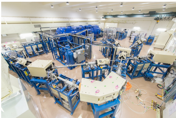
Figure 8: Photograph of the 6 MV Tandem Accelerator System at the University of Tsukuba.
