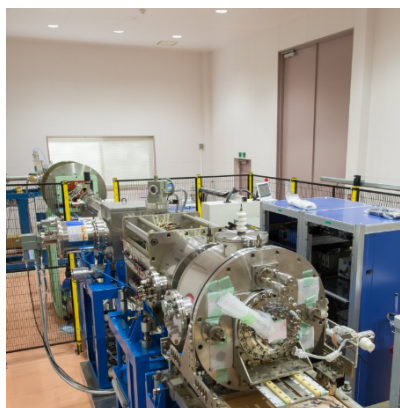
Figure 6: Photograph of the Lamb-shift Type Polarized Ion Source (PIS).
