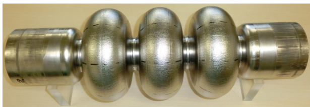
Figure 4: Niobium tube just after hydroforming.
