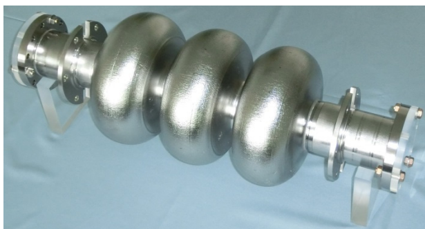
Figure 6: Finished appearance of 3-cell cavity.
