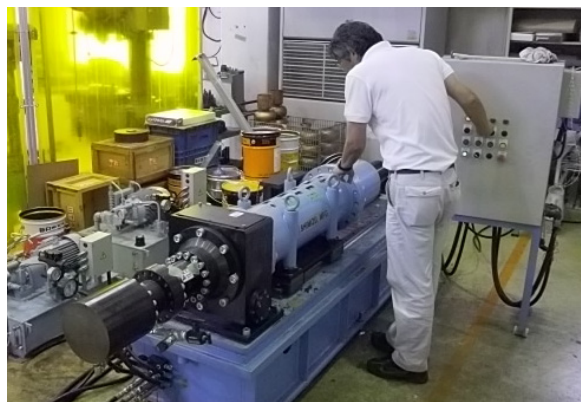
Figure 3: Hydroforming machine (Final hydraulic pressure: 25 MPa).
