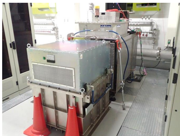
Figure 4: (Upper) PFN charger: type I, and (Lower) type II with the klystron-modulator installed in SACLAL-BL1 linac.
