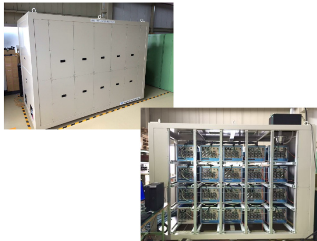
Figure 22: Pulsed power supply as the Klystron Modulator.
