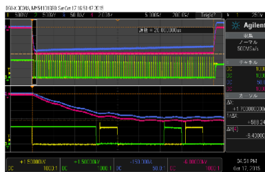
CH1; MARX1 SiC-FET S-D voltage 500V/div CH2; MARX2 SiC-FET S-D voltage 500V/div 5us/div Output voltage rise time (10% -90%): 19us
