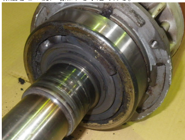
Figure 5: Picture of the damaged pump.
