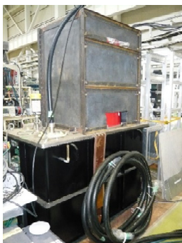
Figure 12: Klystron tank for the TH2104.
