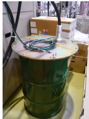
Figure 5: Dummy load for the Chopper-type Marx modulator.
