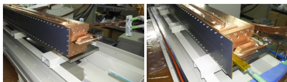
Figure 7: septum I (left) and septum II (right) magnet. Septum II magnet has an extended septum plate and tin vacuum pipe within the gap.
