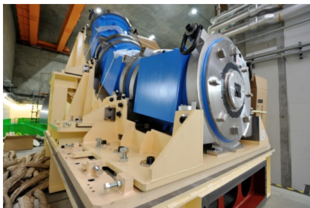
Figure 3: Picture of the superconducting-magnet assembly for (BM01-BM03).
