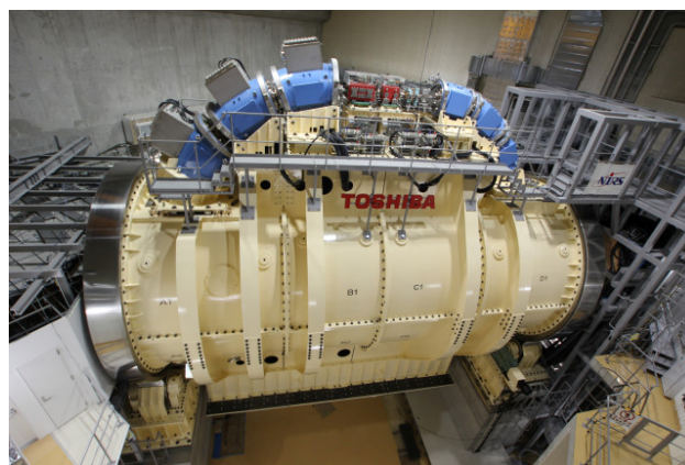
Figure 4: Picture of the superconducting rotating-gantry. A length between the two end rings is 14 m, and the beam orbit radius is 5.45 m.
