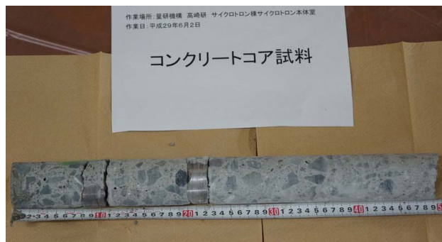
Figure 5: Concrete core of the shielding wall in the cyclotron main room.
