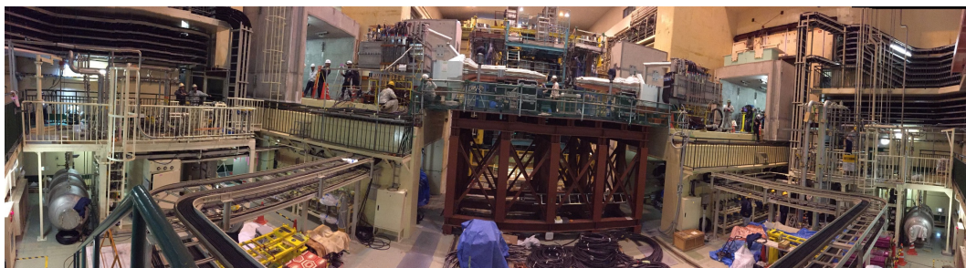
Figure 1: QCS cryostats and cryogenic devices before the Belle II detector roll-in at the Tsukuba experimental hall.
