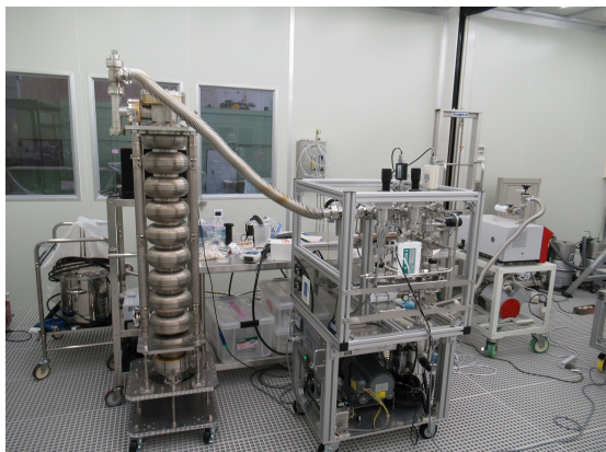
Figure 4: Setup of particle measurement with ERL 9cell cavity by using slow pumping & venting system.
