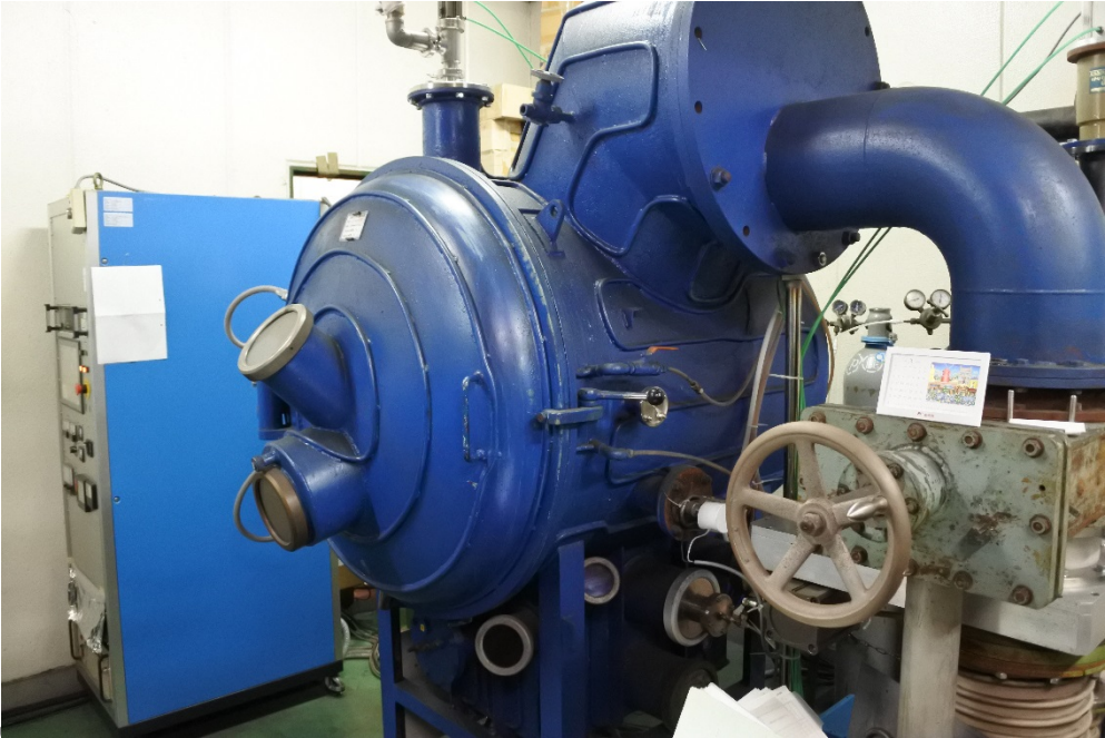
Vacuum furnace for TiN coating @TIGOLD
