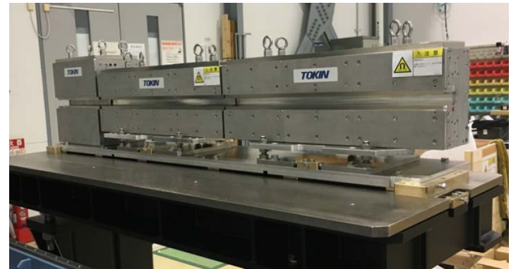
Longitudinal gradient bending (LGB) magnet
