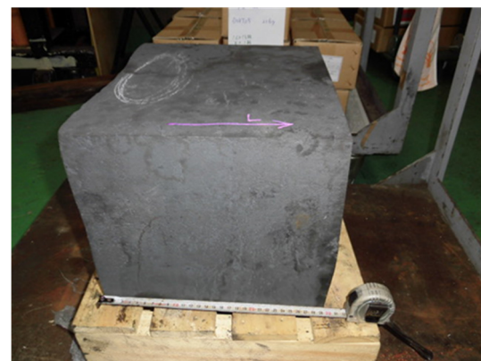
Figure 3: SUS316LN ingot after hot forging treatment.
