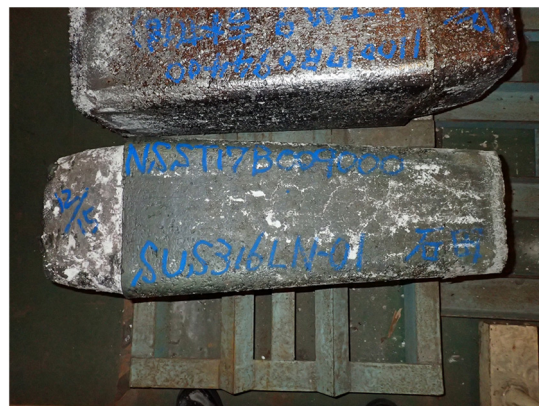
Figure 2: Ingot of SUS316LN after melting (lower ingot).
