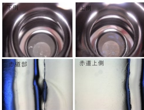
Figure 3: Photos of inner surface after VEP1 (upper) with a digital camera (lower) with Kyoto camera.
