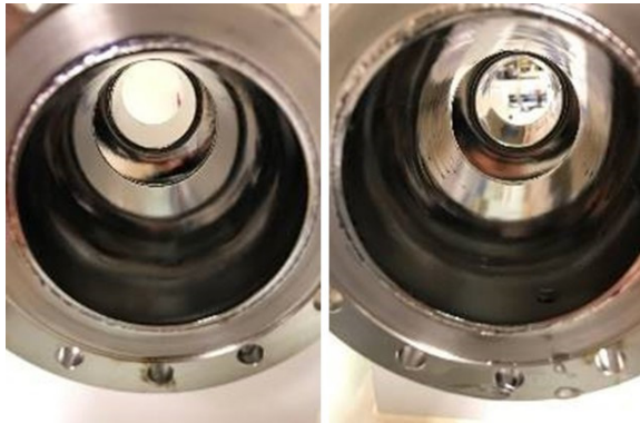
Figure 9: Photos of inner surface after VEP2 with a digital camera.
