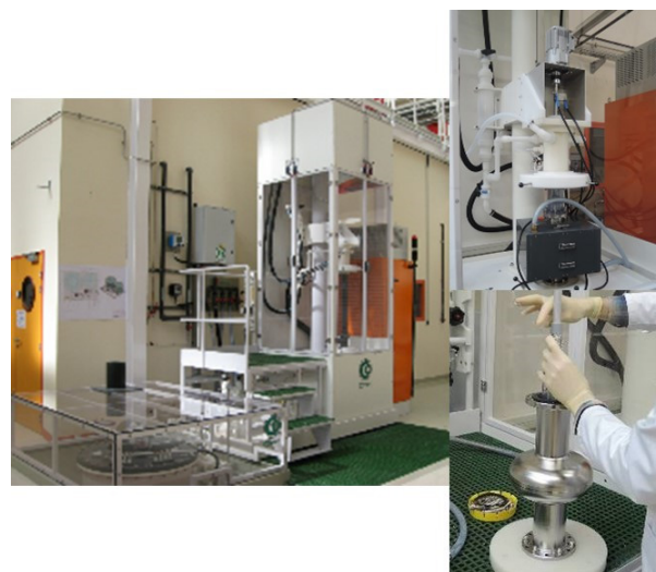
Figure 7: Photos of VEP facility (left), cavity setup (upper right), single cell cavity TP02 (lower right).
