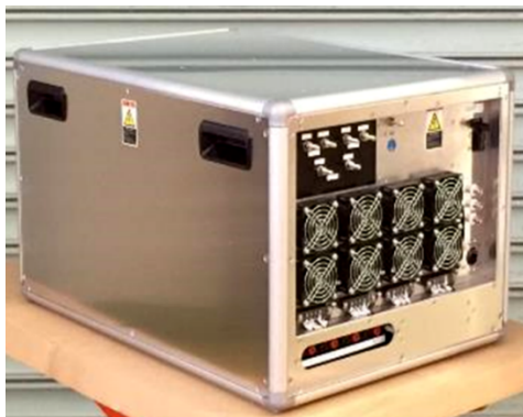
Figure 2: Actual photo of a unit chopper type MARX power supply.
