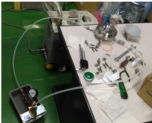
Figure 8: A photo of pressure test and helium leak test.
