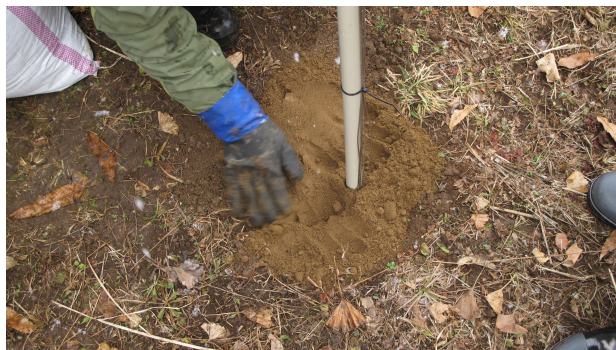
Figure 3: Thermocouples installed in the ground for environment temperature measurement.
