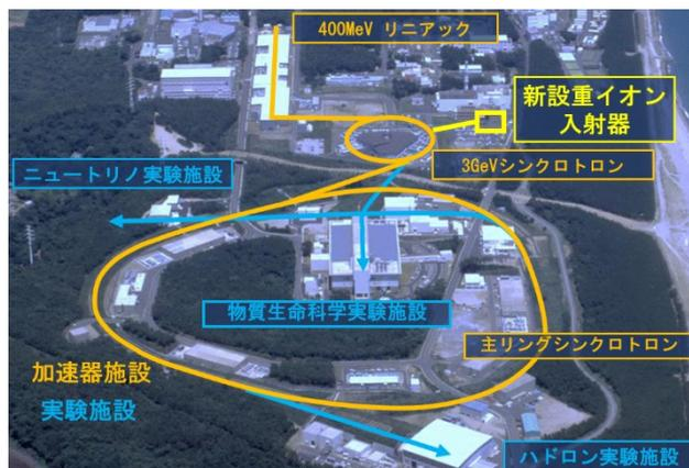
Figure 1: J-PARC facility air photograph. Orange shows accelerators and blue shows experimental facilities. Yellow shows newly planned heavy ion injector.
