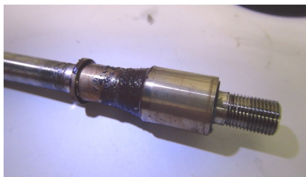
Figure 3: Cuprous oxide attached to the shaft of the flow switch.
