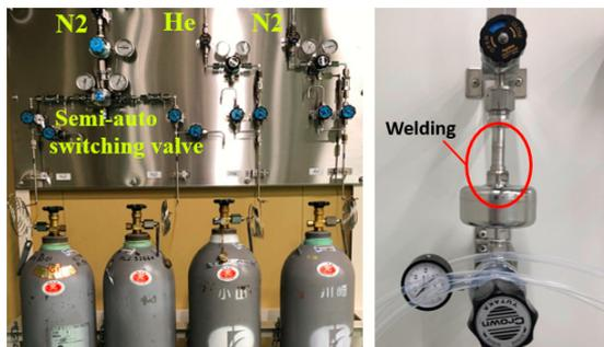
Figure 6: Gas handling panel and gas outlet.
