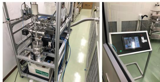
Figure 7: Slow pumping system and operation panel.
