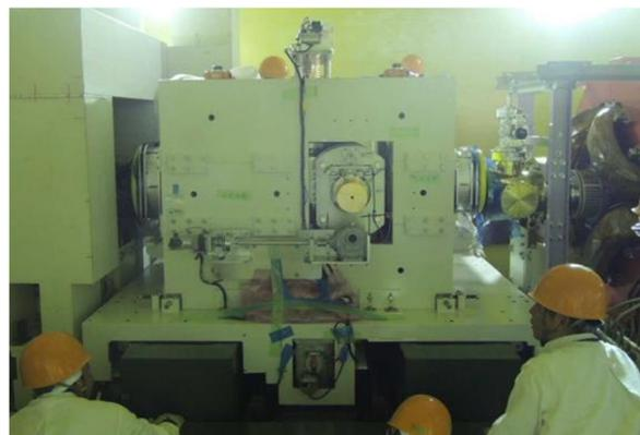
Figure 4: A new collimator with movable blocks.
