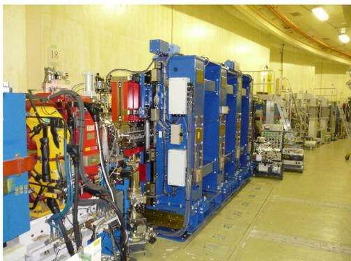
Figure 3: Photograph of new undulator #19 (U#19) after installation into B18-B19 straight section in the PF ring.
