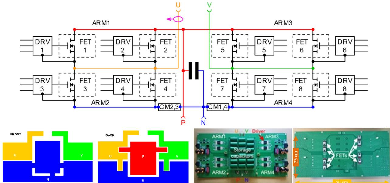
Figure 2: Circuit schematics, structure of buses and picture of the updated design of 4th generation of SPS.
