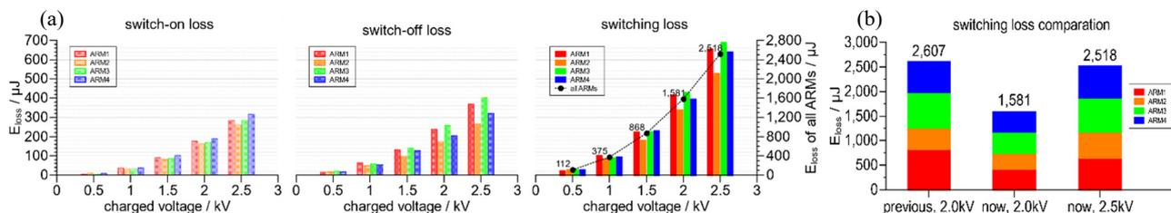
Figure 4: (a) Switch-on loss, switch-off loss and total switching loss of each ARM at different HV. (b) Switching loss comparison of the previous and the updated SPS.
