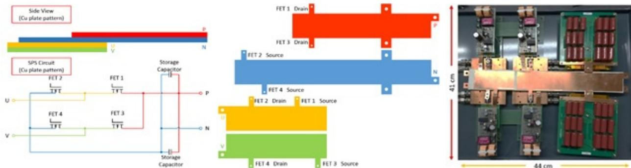
Figure 1: Circuit schematics, structure of buses and picture of the previous design of 4th generation of SPS.
