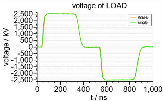
Figure 7: Output voltage of the load at 50 kHz and single shot.
