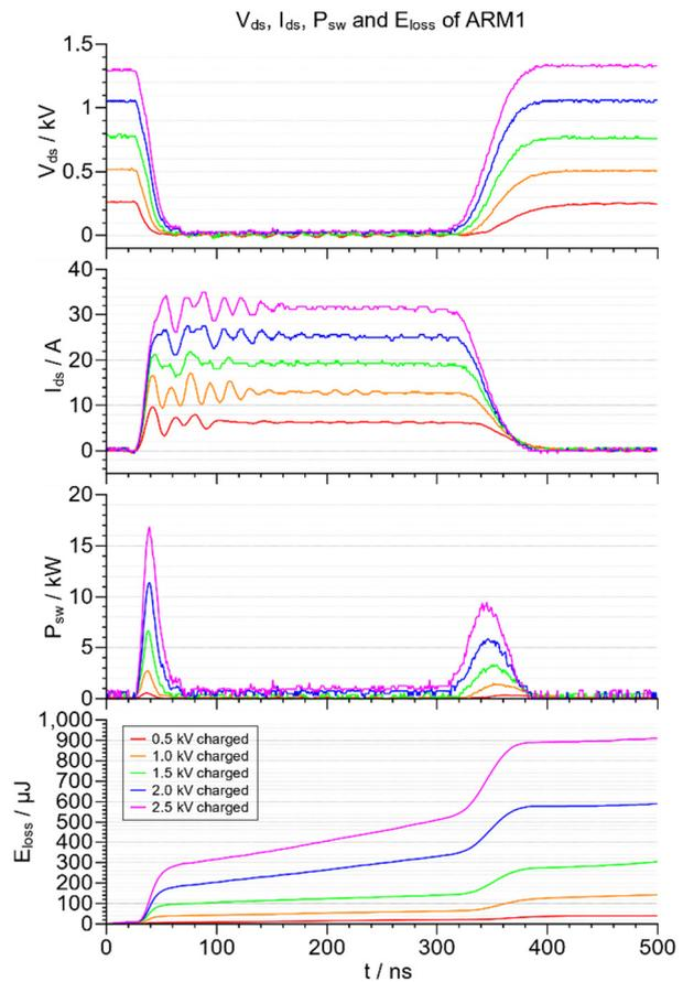
Figure 3:  $V_{ds}$  waveform,  $I_{ds}$  waveform,  $P_{sw}$  and  $E_{loss}$  of ARM 1.
