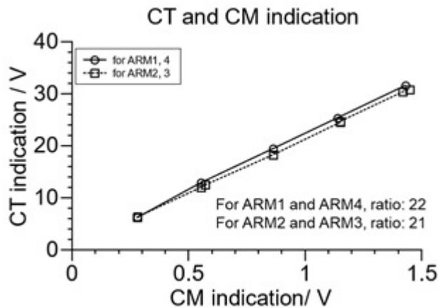
Figure 5: The indications from current transformer and current monitors.
