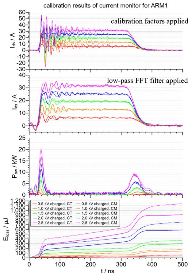
Figure 6: Comparison of the standard waveforms from current transformer and the processed waveforms from current monitor.
