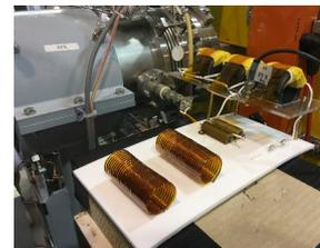
Figure 4: The IT and APN connected to the WERC synchrotron.
