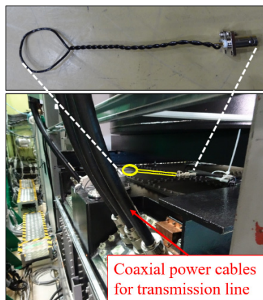
Figure 3: Measurement of common-mode noise with a pickup coil.
